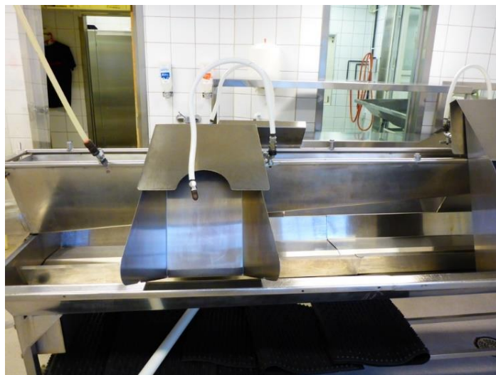
Figure 4 Washing station with filtered water under high pressure. Photo: Henrik A. Kildahl with courtesy from Noraker farm.
