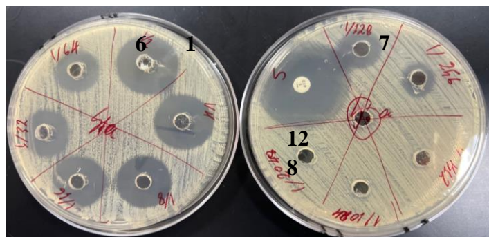
Figure 9 Measurement of MIC for CH-NE-vitE against S. aureus . The designated numbers 1 – 11 represent the serial dilutions from 1/2, 1/4, 1/16, 1/32, 1/64, 1/128, 1/256, 1/512, 1/1024, 1/2048, alongside the 10 µg of the standard antibiotic ciprofloxacin (12).
