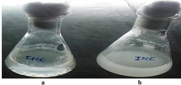
Figure 3 Degradation of oil by (a) immobilized cells and (b) immobilized enzyme
