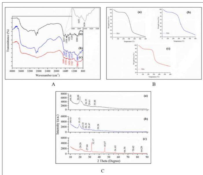
**Figure 6** Characterization of chitosan: Fourier transform infrared spectroscopy (A); Thermogravimetric analysis (B); and X-ray powder diffraction (C). Where (a), chitin; (b) extracted chitosan; and (c) commercial chitosan (Jantzen da Silva Lucas et al., 2021)
