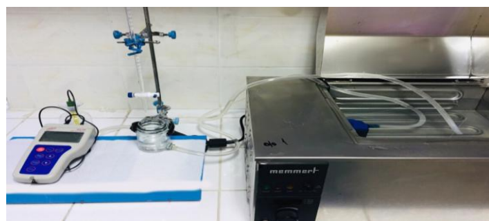
Figure 2 Assay of enzyme activity by using the titrimetric method
