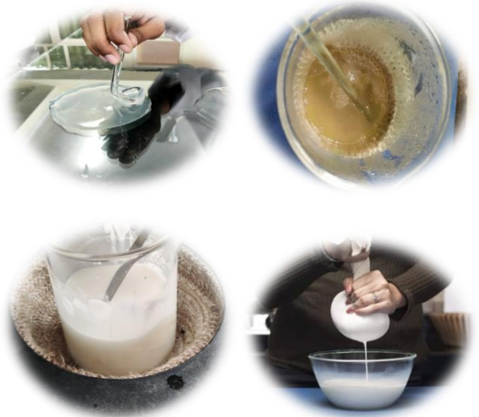
Figure 1 Schematic representation of the development of sago and potato starch-based bioplastic
