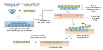
**Figure 2** Schematic representation of the anodic Aluminum Oxide (AAO) membrane used as a 'band-aid technique' for skin tissue engineering. (Poinem Gérrard et al., 2011)
