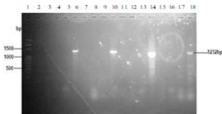
Figure 2 Detection of omt-1 gene; Lane 1, 100bp DNA ladder; Lane 2, negative control 1 (without genomic DNA); Lanes 6, 10, 14, isolates that were positive for omt-1 gene; Lane 17, negative control 2 ( Penicillium fellutanum ATCC 48694); Lane 18 positive control ( Aspergillus flavus ATCC 22546).
