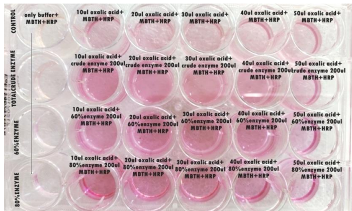
Figure 8 Result layout colorimetric scheme of MBTH based standard H 2 O 2 detection using HRP
