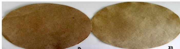
**Figure 12** Pre-bleaching process of Pulp from Waste-paper with ASX42 cellulase-free xylanase. A) Untreated B) Treated with ASX42 cellulase-free xylanase.
