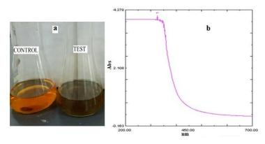
**Figure 1** (a) Reaction vessel containing  $10^{-3}$  M of ferric chloride solution, before reaction (Control) and after 1 hour of reaction at 90°C in water bath (Test). (b) UV-visible absorption spectra of Fe<sub>2</sub>O<sub>3</sub> nanoparticles after 1 hour of reaction
