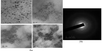
Figure 3 (a) TEM images of synthesized  $Fe_2O_3$  nanoparticles ranging from 5 nm and 50 nm (b) SAED pattern
