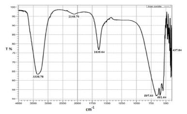
Figure 2 FTIR spectra of Fe<sub>2</sub>O<sub>3</sub> nanoparticles synthesized by neem leaves extract
