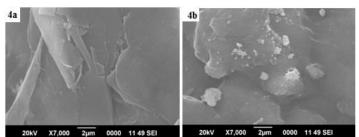
Figure 4 SEM images of  $Fe_2O_3$  nanoparticles uncoated cellulose paper (a) and nanoparticles coated cellulose paper (b)
