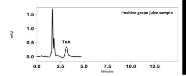
Figure 2 Chromatogram of (a) TeA in aqeous solution, (b) Fruit samples spiked with TeA (c) and a real fruit samples contaminated with TeA (positive sample)
