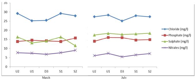
Figure 1 Chloride, nitrate, phosphate and sulphate contents of wastewater in March and July
