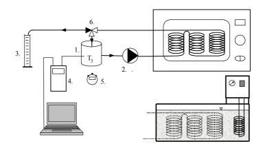
Figure 2 Second version of the heating system. 1-Bottle with juice; 2-Feeding pump; 3-Respective container; 4-ALMENO 2590-9 thermometer; 5-Stopwatch
