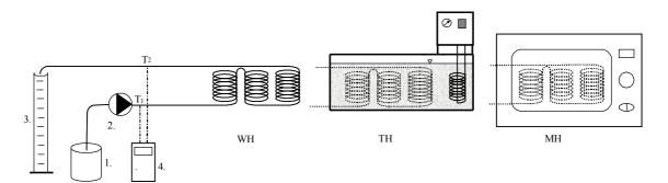
**Figure 1** First version of the heating system 1-Original 5L juice bottle; 2-STENNER 85M5 feeding pump; 3-Respective container; 4-ALMENO 2590-9 thermometer
