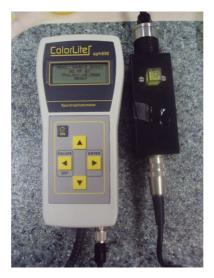
Figure 4 ColorLite sph850 Spectrophotometer in use.
