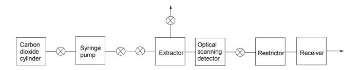
Figure 1 Schematic drawing of SFE apparatus
