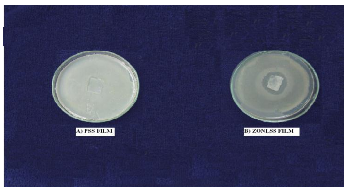
Figure 8 Antimicrobial activity in (A) PSS film (control) (B) ZONLSS film (6% ZnO nanoparticles).
