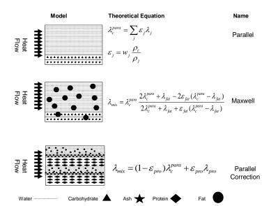
Figure 3 Thermal conductivity model.
