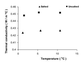
Figure 2 Thermal conductivity of salted and non-salted UF chees
