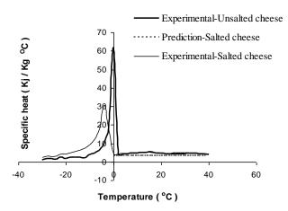
Figure 4 Specific heat values obtained from the DSC and comparison with model
