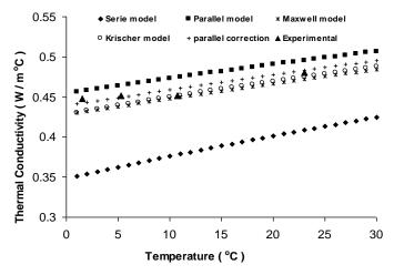
Figure 5 Experimental and predicted thermal conductivity values
