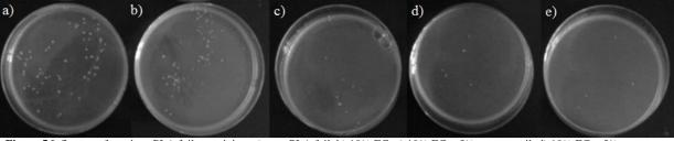
Figure 5 Influence of coatings PLA foil containing: a) pure PLA foil, b) 10% EC, c) 10% EC + 5% caraway oil, d) 10% EC + 5% rosemary oil, e) 10% EC + 5% fennel oil to reduce the number of *S. aureus* cells
