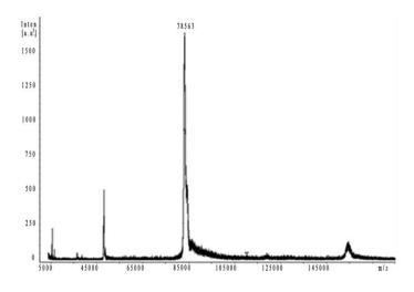
Figure 2 MALDI-TOF analysis to P-80 purified protein. The registered signal corresponds to a molecule with of weight of 78563 Da.
