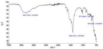
Figure 5 FT-IR Spectrum of ZnO NPs with plant leaf extract of C. alata
