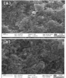
Figure 3 SEM image of ZnO NPs synthesized from *C. alata* leaf extract at different scale bar (a) 2  $\mu$ m (b) 1  $\mu$ m EDX
