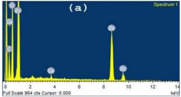
Figure 4 EDX Spectrum of ZnO nanoparticles synthesized from C. alata
