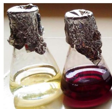
Figure 1 (A) Visual observation of UV-Visible spectra of biosynthesized BPAuNPs (B) Conical flasks confirming BPAuNPs Synthesis
