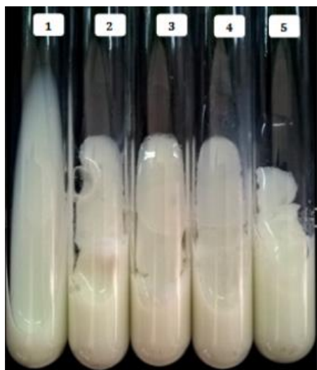
Figure 2 Coagulation of skimmed milk by the crude extract and purified enzyme of M. circinelloides (1: control, 2: crude extract, 3: precipitated pellet with 20-70% (NH 4 ) 2 SO 4 , 4: dialyzed extract, 5: purified enzyme).
