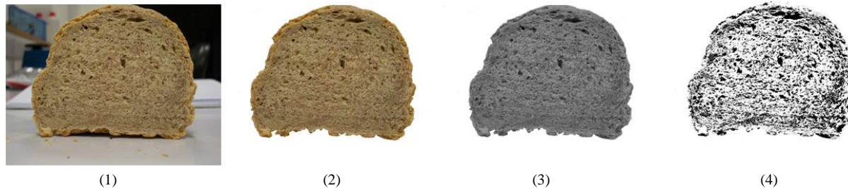
Figure 1 Preparation of bread cross-section image for breadcrumb structure analysis. From left to right: 1) bread cross-section image captured using camera; 2) isolation of bread cross-section using Adobe Photoshop; 3) conversion of image into 8-bit greyscale image using ImageJ software; 4) application of Otsu's thresholding to the 8-bit greyscale image using ImageJ software
