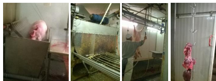
Figure 1 From left: Division of slaughterhouse - part II (steambath and removal of bristles) and part III (evisceration)
